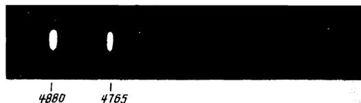
FIG. 3. Radiation spectrum (visible part; chamber of diameter 10 cm).
