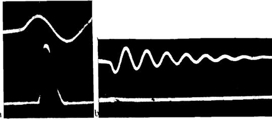
FIG. 4. Oscillograms of current discharge with period of  $\sim 2 \mu\text{sec}$ —upper trace—and generation pulse—lower trace (visible region; chamber of diameter 10 cm): a) electron beam was directed towards the region B (Fig. 1) filled with an initial plasma; b) electron beam was directed towards the high-voltage electrode 4.
