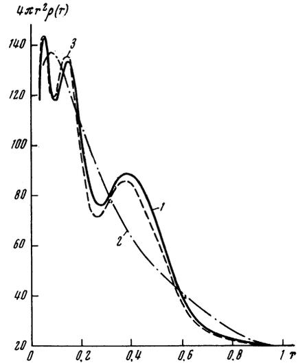
FIG. 3. Radial electron density for the mercury atom: 1—Hartree, 2—Thomas-Fermi, 3—Thomas-Fermi with quantum and oscillator corrections.
