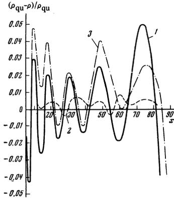
FIG. 2. Relative difference between the quantum-mechanical electron density  $\rho_{qu}$  and the Thomas-Fermi density (1), the density with the oscillatory correction (2), and the density with Troshin's correction [4] (3) for the model of an ideal electron gas in a Coulomb field.
