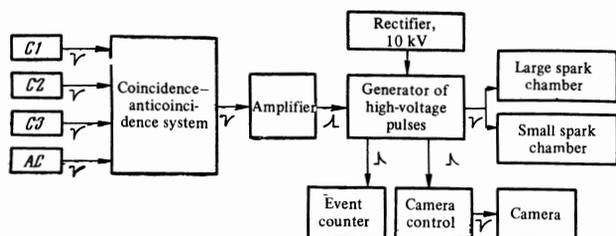
FIG. 4. Block diagram of the electronics.
