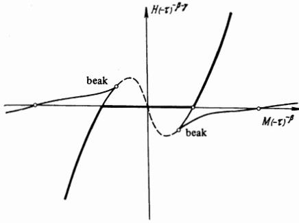
Qualitative form of the isotherm below the Curie point. The thick line is the stable branch, the thin lines are the metastable branches, and the dashed line is the self-consistent field-theory isotherm.
