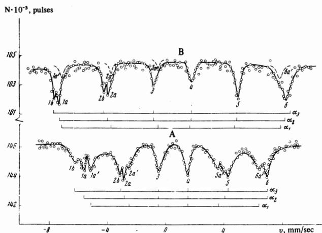
FIG. 1. Mössbauer spectra of a sample of composition 1 subjected to ageing: A) at room temperature; B) at  $T = 196^\circ\text{C}$ . The components denoted by a (continuous curve) and a' (dashed curve) represent inequivalent tetrahedral  $\text{Fe}^{3+}$  ions.
