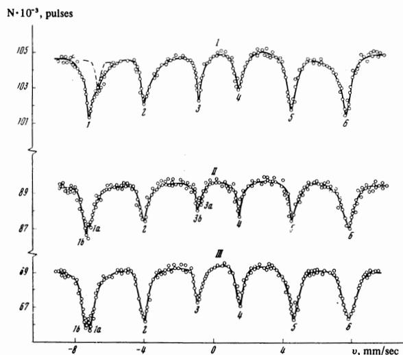
FIG. 2. Mössbauer spectra of a sample of composition 2 subjected to various heat treatments: I) quenching; II) cooling in a switched-off furnace; III) ageing.
