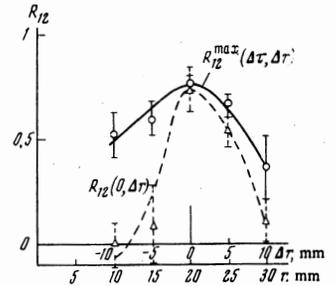
FIG. 6. Correlation function as a function of distance along the radius  $r$ ,  $i = 4\pi/3$ ,  $H_0 = 3$  kOe, solid line— $R_{12}^{\text{max}}(\Delta\tau, \Delta\tau)$ , dashed line— $R_{12}(0, \Delta\tau)$ .
