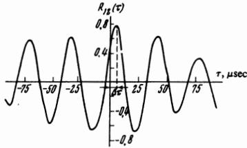
FIG. 5. Correlation function of two signals from probes displaced along a radius by  $\Delta r = 5$  mm.  $i = 4\pi/3$ ,  $H_0 = 3$  kOe.
