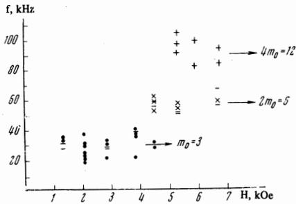
FIG. 7. Frequency and oscillation mode as a function of magnetic field strength  $H_0$ .  $i = 4\pi/3$ ;  $\circ - m_0 = 3$ ;  $\times - 2m_0 = 6$ ;  $+$   $- 4m_0 = 12$ ; the bars denote cases for which determination of the mode was difficult.
