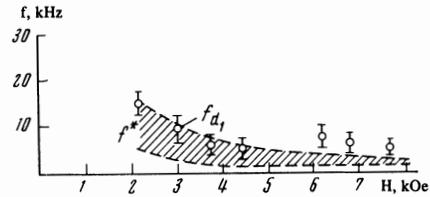
FIG. 8. Oscillation frequency of the first mode  $f_{d1}$  in the coordinate system moving with the plasma, and electron drift frequency  $f^*$  (cross-hatched region), as a function of magnetic field. The value of  $f^*$  was calculated for  $T_e = 2-4$  eV and  $\partial \ln n/\partial r = 0.5-1$   $\text{cm}^{-1}$ .
