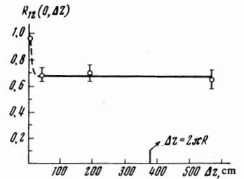
FIG. 4. Correlation function as a function of distance  $\Delta z$  along the magnetic force line.  $i = 4\pi/3$ ,  $H_0 = 3$  kOe.
