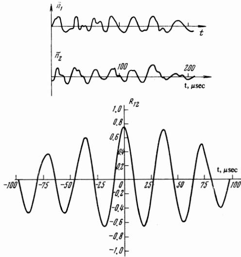
FIG. 3. Oscillograms of oscillations of the saturation ion current to probes located on the same line of force (above), and the mutual correlation function of these signals (below),  $i = 4\pi/3$ ,  $H_0 = 3$  kOe,  $\Delta z = 570$  cm.
