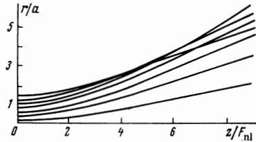
FIG. 1. Aberration picture of the course of the rays of a Gaussian beam in the case of internal defocusing.
