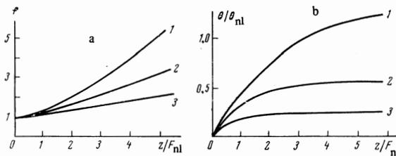
FIG. 2. Solutions of the ray equation, obtained with a computer for different absorptions of the medium: a—trajectory of a beam in a medium with absorptions  $\alpha R_T$  equal to 0, 1, and 9; b—dependence of the nonlinear divergence of the paraxial ray tube on the traversed path in medium with the same absorptions, respectively, for curves 1, 2, and 3.
