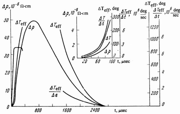
FIG. 1. Variation of the electric resistance, of the effective temperature, and of the rate of heating when beryllium is heated.
