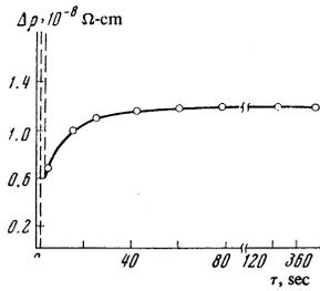
FIG. 3. Change of electric resistance of a sample after irradiation at 77°K.
