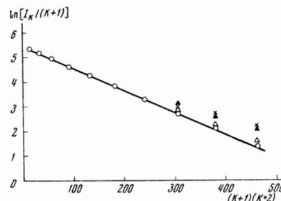
FIG. 1. Graph of Eq. (1) for  $N_2^+$  ions: O—present results, without a metal plate close to the luminous space; X—results in<sup>[4]</sup>;  $\Delta$ —present results, with a steel plate close to the luminous space;  $\blacktriangle$ —the same, with a positive  $\sim 10$ -V potential applied to the steel plate.
