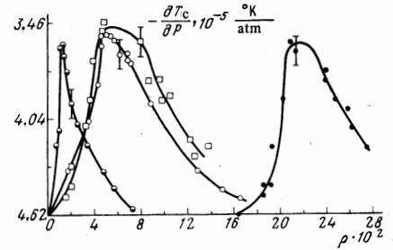
FIG. 7. Dependence of  $\partial T_c/\partial P$  on the relative residual resistivity  $\rho$  on the following systems:  $\circ$ —In-Hg;  $\circ$ —In-Cd;  $\square$ —In-Tl;  $\circ$ —In-Pb2%—Cd.
