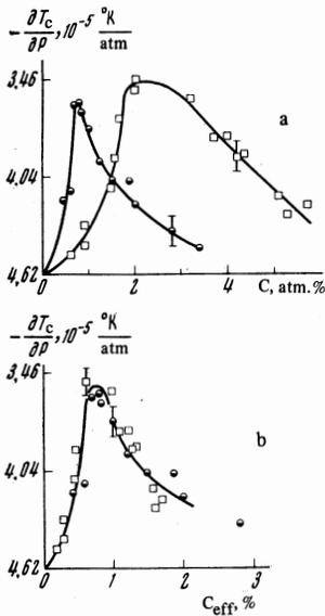
FIG. 6. Dependence of  $\partial T_c/\partial P$  of indium on the impurity concentration (a) and on the effective impurity concentration ( $C_{\text{eff}} = C_{\text{Hg}} = 3.3 C_{\text{Tl}}$ ) (b);  $\bullet$ —In-Hg system;  $\square$ —In-Tl system.
