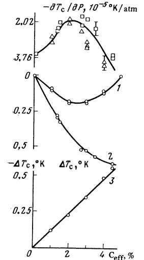
FIG. 10. Dependence of  $\partial T_c / \partial P$  and  $\Delta T_c$  of the alloys In-Tl<sub>35%</sub>-Hg (curve 1) and In-Tl (curve 2) and of the difference of  $T_c$  of the systems In-Tl<sub>35%</sub>-Hg and In-Tl (line 3) on the effective impurity concentration ( $C_{eff} = C_{Hg} = 3.3C_{Tl}$ ).
