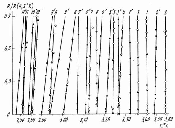
FIG. 1. Temperature dependences of  $R(T)/R(4.2^\circ\text{K})$  for the following systems: 1, 1'-pure In; 2, 2'-In-Hg (8%); 3, 3'-In-Hg (0.8%); 4, 4'-In-Tl (26%); 5, 5'-In-Hg (10%); 6, 6'-In-Tl (3%); 7, 7'-In-Tl (35%); 8, 8'-In-Tl (35%)-Hg (4%); 9, 9'-In-Tl (35%)-Hg (2%); 10, 10'-In-Tl (45%); 11, 11'-In-Tl (50%). Curves 1-11 were plotted at  $P = 0$  and 1'-11' at  $P = 1730$  atm.
