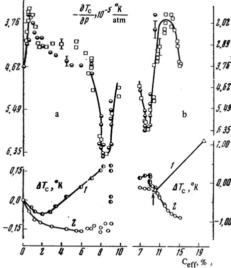
FIG. 9.  $\partial T_c / \partial P$  and  $\Delta T_c$  of the alloys In-Hg and In-Tl vs. the effective impurity concentration ( $C_{eff} = C_{Hg} = 3.3C_{Tl}$ ). a—face centered tetragonal phase; the arrow corresponds to the phase transition, b—Face-centered cubic phase.
