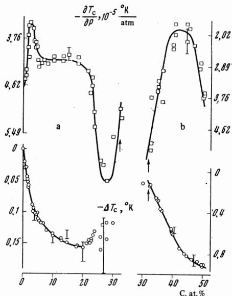
FIG. 2. Plots of  $\partial T_c / \partial P$  and  $\Delta T_c$  of In-Tl alloys against the Tl impurity concentration: a—face-centered tetragonal phase; the arrow corresponds to the phase transition; b—face-centered cubic phase. (The data of [7] are given together with the limits of the errors).
