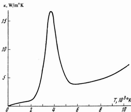
FIG. 5. Temperature dependence of the thermal conductivity of hydrogen at atmospheric pressure.
