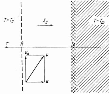
FIG. 11. Diagram of planar discharge in a gas stream. The dashed line represents a grid cooled to a temperature  $T_0$ . The doubly-hatched region corresponds to the transition layer on the discharge boundary.
