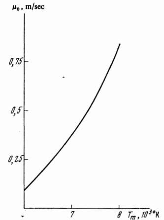
FIG. 12. Dependence of the velocity of the free propagation of the discharge in hydrogen at atmospheric pressure.
