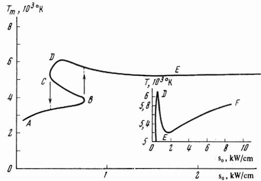
FIG. 6. Dependence of the temperature on the discharge axis on the power for hydrogen at atmospheric pressure.  $R = 10$  cm,  $\omega = 10^{10}$  sec $^{-1}$ .
