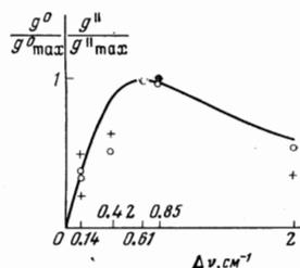
FIG. 2. Dependence of the relative amplification coefficient for circular ( $\circ - g^0(\Omega)/g_{\text{max}}^0$ ) and linear ( $+ - g''(\Omega)/g_{\text{max}}''$ ) polarizations of the exciting radiation. The continuous curve is the theoretical curve. To the given measurements one should add the quantity  $g^0/g_{\text{max}}^0 = g''/g_{\text{max}}'' = 0.96$  for  $\Delta\nu = 0.54 \text{ cm}^{-1}$ .
