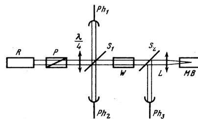
FIG. 1. Arrangement of apparatus for the measurement of the amplification coefficient of the SRW. R—Ruby laser, P—Glan prism,  $S_1$ ,  $S_2$ —separating plates,  $Ph_1$ ,  $Ph_2$ ,  $Ph_3$ —radiation detectors,  $W$ —vessel with test liquid,  $L$ —focusing lens,  $MB$ —SMBS generator.
