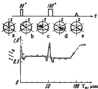
FIG. 2. Nuclear spin echo signal intensity following the action of 90 and  $180^\circ$  rf pulses against the delay time ( $T_p$ ) of the start of the microwave pulse relative to the start of the rf pulse.  $P/P_{\text{thr}} = 10$  dB ( $P_{\text{thr}}$ —threshold excitation power of parametric spin waves),  $H_0 = 1050$  Oe. Top (a–e)—diagrams illustrating the formation of the nuclear spin-echo signal following the action of 90 and  $180^\circ$  rf pulses.
