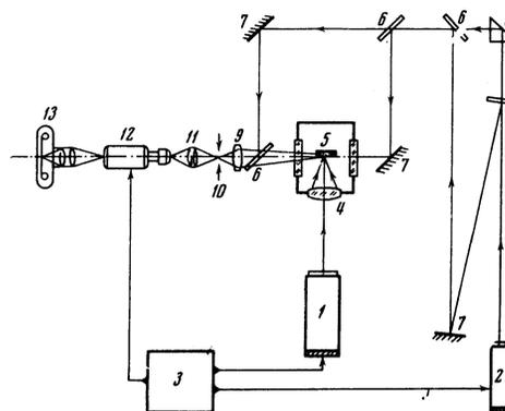
FIG. 1. Diagram of a setup for time scan of flare interferogram using an image converter. 1—neodymium laser; 2—ruby laser; 3—control unit; 4—focusing lens; 5—target; 6—beam splitters; 7—mirrors; 8—prism; 9—lens for projecting interference image on the slit; 10 and 11—lens for projecting slit image on photocathode; 12—photoelectric recorder; 13—camera.
