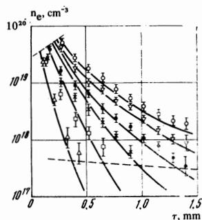
FIG. 3. Electron density distribution along the axis of a laser beam at various times reckoned from the beginning of the laser pulse (in nanoseconds):  $\Delta$ — $t = 10$ ;  $\square$ — $t = 16$ ;  $\times$ — $t = 23$ ;  $\bullet$ — $t = 36$ ;  $\nabla$ — $t = 56$ ;  $\circ$ — $t = 76$ .
