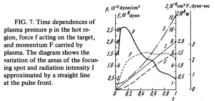
FIG. 7. Time dependences of plasma pressure  $p$  in the hot region, force  $f$  acting on the target, and momentum  $F$  carried by plasma. The diagram shows the variation of the areas of the focusing spot and radiation intensity  $I$  approximated by a straight line at the pulse front.
