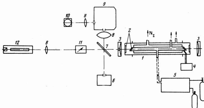
FIG. 4. Setup for ruby laser measurements. 1—cell cooled with liquid nitrogen; 2—CaF<sub>2</sub> windows; 3—mirrors; 4—thermocouple; 5—gas feed system; 6—IEK-1 calorimeter; 7—plane parallel plate; 8—lenses; 9—IKM-1 monochromator; 10—GeAu detector; 11—KDP crystal; 12—ruby laser.
