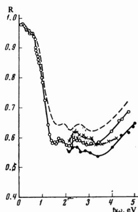
FIG. 1. Reflectivity of molybdenum is given by different workers.  $\circ$ —Mo(100), present paper, dashed—mechanically polished (MP) sample [1,2];  $\times$ —MP sample annealed in vacuum  $10^{-7}$  mm Hg at  $T = 2200^\circ\text{K}$  [3];  $\bullet$ —MP sample annealed in vacuum [4].
