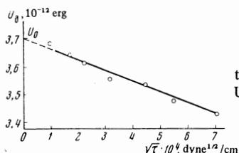
FIG. 3. Dislocation motion activation energy as the function  $U_d(\sqrt{\tau})$ .
