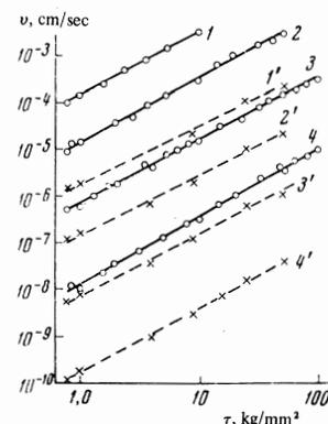
FIG. 1. Dependence of the velocity of individual dislocations  $v$  on the tangential stresses  $\tau$  in undoped silicon at temperatures 800° (1, 1') 700° (2, 2'), 600° (3, 3') and 500°C (4, 4'). The solid lines (1–4) denote the experimental results:  $m_1 = 1.30$ ,  $m_2 = 1.33$ ,  $m_3 = 1.35$ ,  $m_4 = 1.43$ . The dashed curves (1'–4') describe the results of calculations by formula (7):  $m_1' = 1.28$ ,  $m_2' = 1.30$ ,  $m_3' = 1.33$ ,  $m_4' = 1.38$ .
