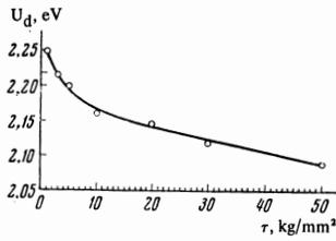
FIG. 2. Dependence of the activation energy of the dislocation motion  $U_d$  on the stress  $\tau$  (experimental data).
