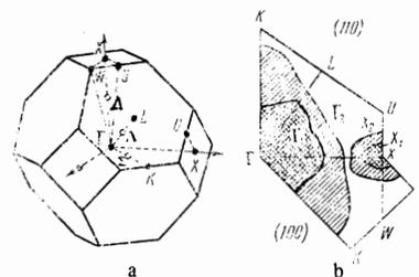
Brillouin zone for FCC metals (a) and cross sections of the Fermi surface of iridium for the (100) and (111) planes according to calculations<sup>[2]</sup> (b).
