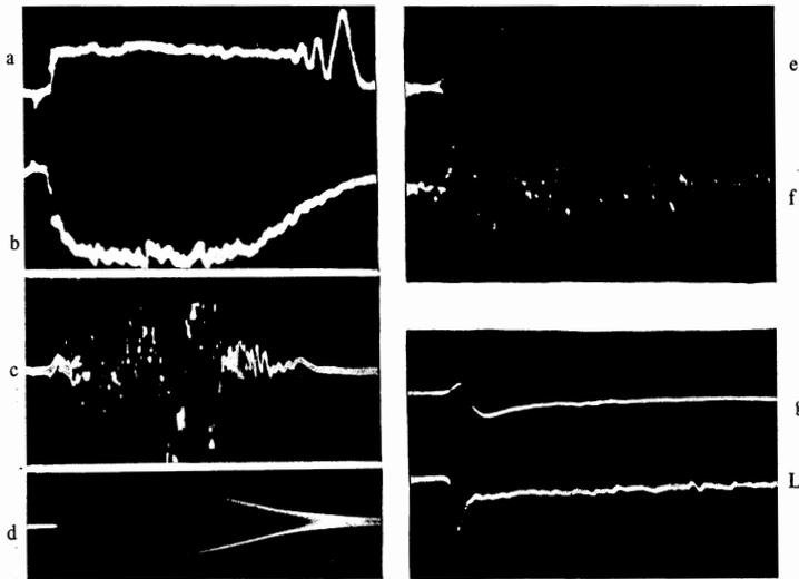
FIG. 1. a—Output of the 2.26-mm interferometer, b—intensity of the continuum between 5700 and 5750Å, c—reflected 2.26-mm signal, d—signal of the Rogowski loop measuring the current in the plasma, e—magnetic probe output, f—rectified magnetic probe output, g—low-frequency component of the diamagnetic probe, h— $H_{\beta}$ . Time scale a–d 500  $\mu$ sec, e–h 200  $\mu$ sec.
