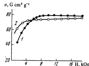
FIG. 4. Dependence of the specific magnetization on the field at  $20^\circ\text{C}$  (curve 1) and at  $124^\circ\text{C}$  (curve 2).
