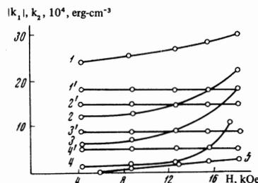
FIG. 2. Dependence of the anisotropy constants  $K_1$  and  $K_2$  on the external field for various temperatures: 1 and 1', 90°C; 2 and 2', 105°C; 3 and 3', 114°C; 4 and 4', 125°C; 5, 137°C (the primed numbers refer to  $K_2$ ).
