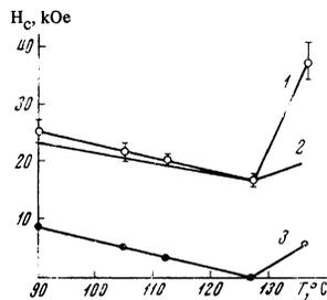
FIG. 3. Dependence of the critical field (curves 1 and 2) and of the anisotropy field (curve 3) on temperature (curve 2 calculated by formula (4)).
