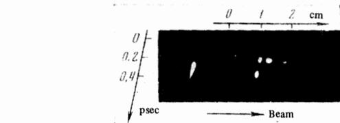
FIG. 3. Photograph taken from the image-converter screen showing the time and space distribution of points of nonlinear scattering of laser radiation in air at atmospheric pressure. An interference filter transmitting at the ruby laser wavelength was placed in front of the image-converter objective. The laser pulse is on the left of the photograph.
