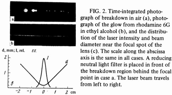
FIG. 2. Time-integrated photograph of breakdown in air (a), photograph of the glow from rhodamine 6G in ethyl alcohol (b), and the distribution of the laser intensity and beam diameter near the focal spot of the lens (c). The scale along the abscissa axis is the same in all cases. A reducing neutral light filter is placed in front of the breakdown region behind the focal point in case a. The laser beam travels from left to right.
