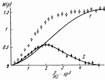
Momentum distribution of parapositronium atoms: O—experimentally obtained total momentum distribution  $L(p)$ ; ●—experimentally obtained momentum distribution of parapositronium atoms  $N(p)$  (the narrow component of the correlation curve). 1—curve for the broad component  $M(p)$  calculated by the Coulson-Duncanson method; 2—momentum distribution curve for parapositronium atoms calculated from Eq. (6).
