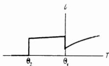
FIG. 4. Dependence of the specific heat  $C$  of Rochelle salt on temperature  $T$ .
