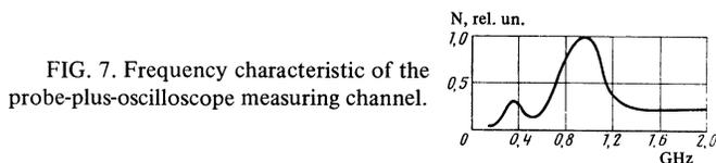
FIG. 7. Frequency characteristic of the probe-plus-oscilloscope measuring channel.
