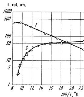
FIG. 6. Temperature dependence of  $I_e$  (curve 1) and  $I_C$  (curve 2) for a sample of pure silicon excited with a laser.
