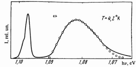
FIG. 3. Spectral distribution of the laser-excited recombination radiation of pure silicon ( $\rho \approx 3 \times 10^4 \text{ ohm-cm}$ ) at  $4.2^\circ\text{K}$ , accompanied by emission of a TO phonon. The spectrum calculated from formula (5) for  $n_0 = 3.7 \times 10^{18} \text{ cm}^{-3}$  is represented by the circles.
