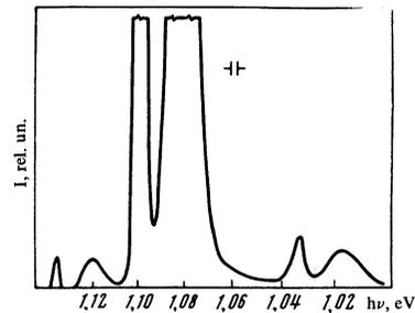
FIG. 1. Spectral distribution of recombination radiation of pure silicon at  $T \approx 10^2 \text{ K}$  and under electron excitation (15 kV, 0.5 mA, pulse duration 5  $\mu\text{sec}$ ).
