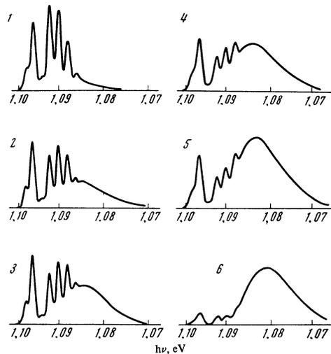
FIG. 8. Change of recombination-radiation spectra of silicon with  $N_B = 5 \times 10^{12} \text{ cm}^{-3}$  with changing laser focusing. The excitation density increases from spectrum 1 to spectrum 6. Temperature 2°K.
