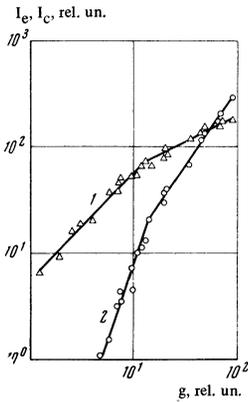
FIG. 5. Dependence of  $I_e$  (curve 1) and  $I_C$  (curve 2) of the sample of pure silicon on the excitation rate  $g$  at 4.2°K.
