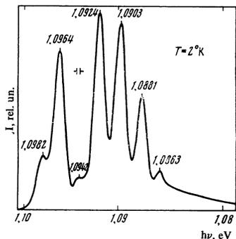
FIG. 7. Spectral distribution of TO component of the recombination radiation of silicon doped with boron ( $N_B = 5 \times 10^{12} \text{ cm}^{-3}$ ) at 2°K and under excitation with defocused laser radiation.
