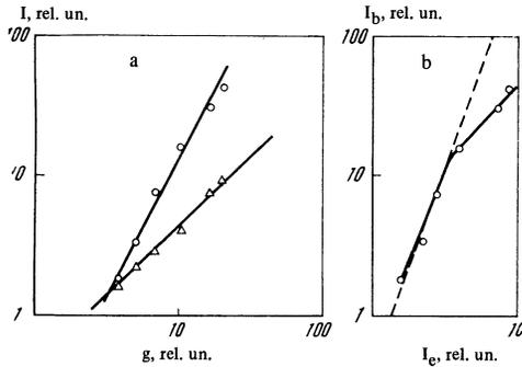
FIG. 2. a—Radiation intensity of free excitons,  $I_e$ , and of the long-wave radiation,  $I_b$ , vs. the excitation rate  $g$  [4]. b—Dependence of  $I_b$  on  $I_e$ , plotted by us from the data of Haynes [4].  $\Delta$ —exciton,  $\circ$ —biexciton,  $T \sim 3^\circ\text{K}$ .
