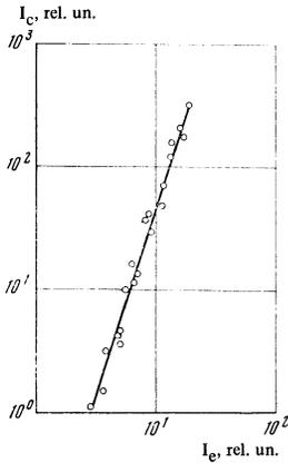
FIG. 4. Dependence of  $I_C$  on  $I_e$  for pure silicon ( $\rho \approx 3 \times 10^4$  ohm-cm) at 4.2°K and laser excitation.
