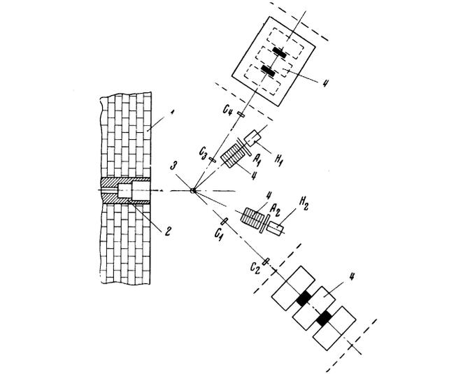
FIG. 2. Experimental setup: 1) Shield, 2) collimator, 3) scatterer, 4) spark chambers,  $C_1 - C_4$ ) proton counters,  $H_1, H_2$ ) neutron counters,  $A_1, A_2$ ) anticoincidence counters.
