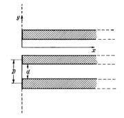
The problem is solved in the hydrodynamic approximation, which can be used if the free path length l of the elementary excitations (phonons and rotons) is much smaller than the capillary width d ( $l \ll d$ ). The width of the capillaries, according to the conditions of propagation of fourth sound, should be much smaller than the viscous wavelength  $\lambda_{\rm V} = \sqrt{2 \eta / \omega \rho_{\rm n}}$  ( $\eta$  is the viscosity of the normal component,  $\omega$  the sound frequency):
