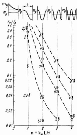
FIG. 6. Relative intensity of the excitation of various spin-wave modes in films of different thicknesses in the absence of the surface pinning of spins. The film thickness is given in terms of the skin depth under resonance conditions.
