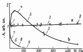
FIG. 1. NMR signal amplitude  $A$  against the intensity of the constant field  $H$  and its direction relative to the RF field  $h$  in the (111) plane: a— $H \perp (111)$ ,  $h \parallel (111)$ ; b— $(H \parallel (111))$ ; c— $(H \perp h) \parallel (111)$ . The amplitude  $A$  for the demagnetized state is arbitrarily taken to be unity. The numbers denote the states for which the DBR spectra are shown in Fig. 2.
