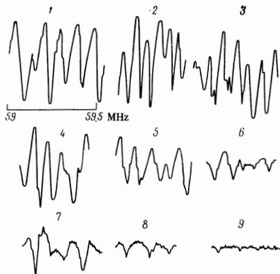
FIG. 2. DBR spectra for hematite in the 59-MHz region for the states correspondingly numbered in Fig. 1.
