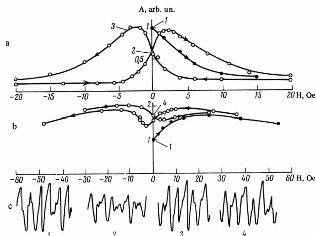
FIG. 3. Hysteresis of the NMR signal amplitude  $A$  for hematite in weak fields: a— $(H \parallel h) \parallel (111)$ ; b— $(H \perp h) \parallel (111)$ ; c—DBR spectra near 59 MHz for the states correspondingly numbered on the hysteresis curves. The amplitude  $A$  for the demagnetized state is taken to be equal to unity.
