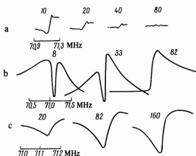
FIG. 5. Examples of NMR signals recorded with the aid of magnetic modulation at different amplitudes and directions of the alternating field  $\mathcal{H}$ : a—( $\mathcal{H} \parallel \mathbf{h}$ )  $\parallel$  (111); b—( $\mathcal{H} \perp \mathbf{h}$ )  $\parallel$  (111); c— $\mathcal{H} \perp$  (111),  $\mathbf{h} \parallel$  (111). The numbers over the curves denote the maximum value of the alternating field  $\mathcal{H}$  in Oe.
