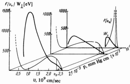
FIG. 2. Longitudinal-velocity distribution function  $f(v_{||})$  (thin curves) and average transverse beam-electron energy  $W_{\perp}$  (thick curves);  $v_0$  is the average velocity of the unperturbed beam.
