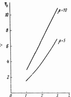
FIG. 3. The dependence of the stabilizing modulation coefficient  $\eta_S = E_S/E_C$  on the effective length of the sample  $l = (1 + y^2)^{-1/2} L/a$ .
