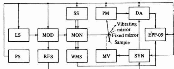
FIG. 1. Block diagram of the apparatus used in the measurements in the 1.5–5.5 eV energy range: LS is the source of light; MOD—modulator; RFS—reference frequency source; SS—spectral scanning device; MON—monochromator of the SPM-2 type; WMS—wavelength-mark source; PM—photomultiplier; DA—detector-amplifier unit; SYN—synchronizer; MV—mirror vibrator (the double-headed arrow indicates the directions of the vibrations of the movable mirror); PS—power source.
