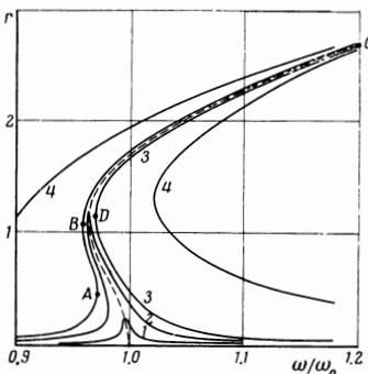
FIG. 1. Dependence of  $r$  on the frequency ratio  $\omega/\omega_0$  for different values of the Q-switching amplitude  $\xi$ : 1- $\xi = 2 \times 10^3 \text{ sec}^{-1}$ , 2- $\xi = 10^4 \text{ sec}^{-1}$ , 3- $\xi = 2 \times 10^4 \text{ sec}^{-1}$ , 4- $\xi = 10^5 \text{ sec}^{-1}$ .
