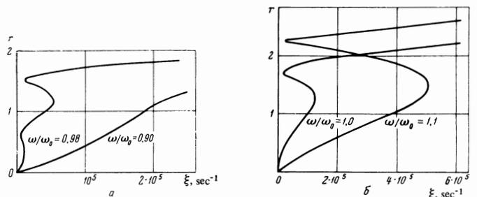
FIG. 2. Dependence of  $r$  on the Q-switching amplitude  $\xi$  at different frequencies  $\omega/\omega_0$ .
