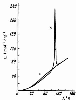
FIG. 1. Specific heat of magnetic specimens with different density of structural vacancies as a function of temperature. a) Density of vacancies  $\sim 4$  at. %; b) density of vacancies  $\sim 1\%$ .
