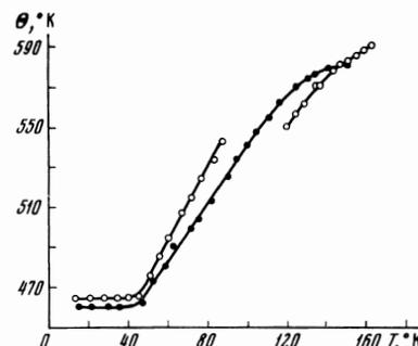
FIG. 3. Temperature dependence of the Debye temperature  $\Theta_D$  on  $T$  for magnetite specimens:  $\circ$ —density of vacancies  $\sim 4$  at. %;  $\square$ —density of vacancies  $\sim 1$  at. %.
