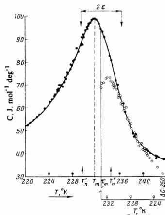
FIG. 5. Specific heat of vanadium deuteride [1] as a function of temperature in the region of the singularity.  $\bullet$ -experimental;  $\circ$ -mirror reflection in  $\tau_m$  and values of the specific heat on the left-hand branch shifted by  $\Delta C$ .
