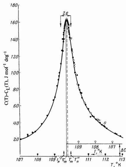
FIG. 2. Specific heat of magnetite in the region of the singularity as a function of temperature: ●—experimental values; ○—mirror reflection in  $\tau_m$  and values of the specific heat on the left-hand branch shifted by  $\Delta C$ .
