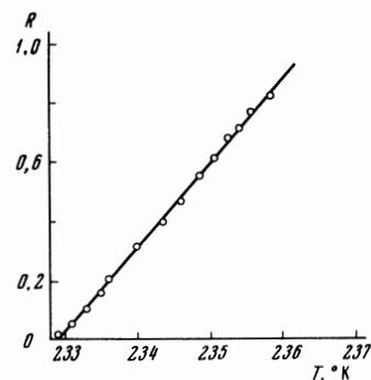
FIG. 6. The quantity  $R = [(C_-(t) - C_+(t))/\Delta C]^{1/2}$  in Fig. 5 as a function of temperature for vanadium deuteride [1] in the region  $(\tau_m, \tau_m + \epsilon)$ .
