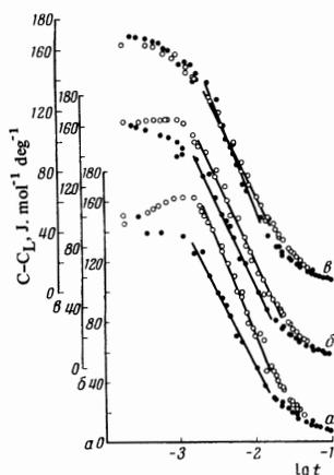
FIG. 4. Specific heat ( $C - C_L$ ) as a function of  $\log t$  for magnetite: a- $\tau_m = 109.66^\circ\text{K}$ ; b- $\tau_m = 109.72^\circ\text{K}$ ; c- $\tau_m = 109.78^\circ\text{K}$ ;  $\bullet$ - $T < \tau_m$ ,  $\circ$ - $T > \tau_m$ .
