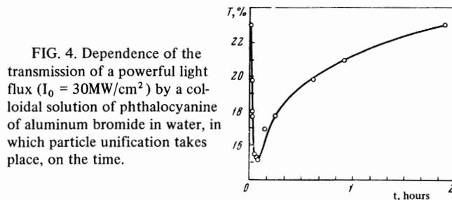
FIG. 4. Dependence of the transmission of a powerful light flux ( $I_0 = 30 \text{ MW/cm}^2$ ) by a colloidal solution of phthalocyanine of aluminum bromide in water, in which particle unification takes place, on the time.
