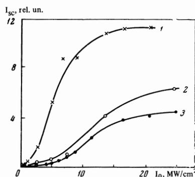
FIG. 3. Dependence of the light scattered at 90° on the intensity of the incident radiation for the following colloidal solutions: 1—adducts of phthalocyanine of aluminum chloride with aluminum bromide in dichlorobenzene, 2—2, 3-naphthalocyanine of copper in quiniline, 3—1, 2-naphthalocyanine of platinum in quiniline.
