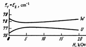
FIG. 7. Dependence of the frequencies of the spin-wave spectrum on the intensity of the external magnetic field  $H \parallel x$  for the points W and U of the magnetic Brillouin zone of  $\text{KMnF}_3$ .
