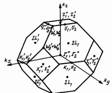
FIG. 6. Irreducible representations of excitons and magnons for symmetric points of the Brillouin zone of  $\text{KMnF}_3$ , consistent with the corresponding representations at the point  $\Gamma(0,0,0)$  for the case when the magnetic moment is parallel to the  $x$  axis of the crystal.
