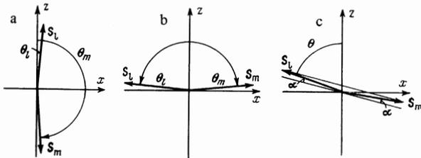
FIG. 4. Possible configurations with a weak magnetic moment for  $\text{KMnF}_3$  in the absence of an external magnetic field: a -  $\theta_l + \theta_m = \pi \tan(\theta_l - \theta_m) = A_2/(12J_{12} + A_1)$ ; b -  $\theta_l + \theta_m = 0$ ,  $\tan(\theta_l - \theta_m) = -A_2/(12J_{12} - A_1)$ . Case c - rotation of the magnetic moments of the sublattices from the configuration b in an external magnetic field parallel to the  $x$  axis.
