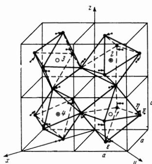
FIG. 1. Distortions of the fluorine octahedra for four neighboring  $Mn^{2+}$  ions in the  $KMnF_3$  lattice;  $\circ$  and  $\odot$  —  $Mn^{2+}$  ions with spin orientations — and + respectively;  $\bullet$  —  $F^-$  ions;  $\eta = 0.060a$ ,  $\epsilon = 0.05a$ ,  $\xi = 0.06a$ .<sup>[3]</sup>
