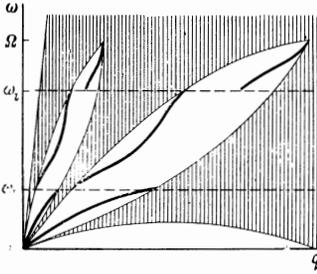
FIG. 2. Dispersion curves in a leaf-type "window."
