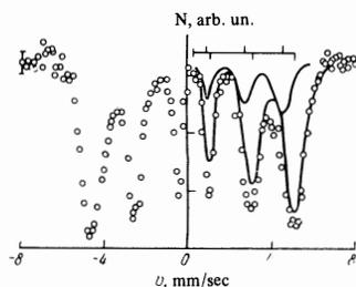
FIG. 1. Mossbauer spectrum of  $\text{Fe}^{57}$  nuclei in the ferrite  $\text{Li}_{0.5}\text{Fe}_{1.1}\text{Cr}_{1.4}\text{O}_4$  at  $T = 293^\circ\text{K}$ .
