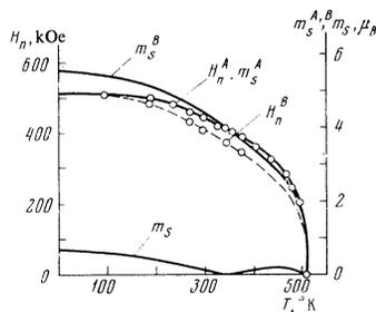
FIG. 5. Temperature dependence of the quantities H<sub>n</sub><sup>A</sup>, H<sub>n</sub><sup>B</sup>, m<sub>S</sub><sup>A</sup>, m<sub>S</sub><sup>B</sup> and m<sub>S</sub> for Li<sub>0.5</sub>Fe<sub>1.3</sub>Cr<sub>1.2</sub>O<sub>4</sub>.
