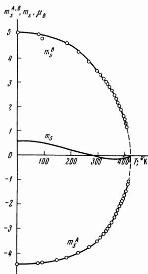
FIG. 4. Dependences  $m_S^A(T)$  and  $m_S^B(T)$  (from data of Mossbauer effect measurements) and  $m_S(T)$  (from data of measurements of the magnetic moment) for  $\text{Li}_{0.5}\text{Fe}_{1.1}\text{Cr}_{1.4}\text{O}_4$ .
