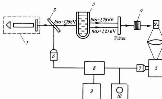
FIG. 1. Scheme of the experimental setup. 1 – Ruby laser; 2 – glass deflecting plate; 3 – Dewar flask with liquid nitrogen; 4 – attenuator for exciting light; 5 – MDR-2 monochromator; 6, 7 – photodiodes; 8 – synchronous pulse detector; 9 – ÉPP-09 automatic recorder; 10 – long-persistence oscillograph.
