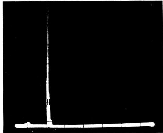
FIG. 5. Beat signal when the distance between the laser mirror and the object is an integer multiple of the resonator length.
