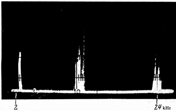
FIG. 4. Beat signals at frequencies  $\Delta\nu_{3.39} = 2.2\ \text{kHz}$ ,  $2\Delta\nu_{3.39} = 4.4\ \text{kHz}$ ,  $\Delta\nu_{0.62} = 12\ \text{kHz}$ , and  $2\Delta\nu_{0.63} = 24\ \text{kHz}$ .
