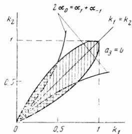
FIG. 9. Stability diagram of stimulated oscillations in a laser.
