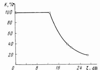
FIG. 6. Depth of modulation  $K$  of the laser radiation against the attenuation of the intensity of the back signal  $\xi$ .
