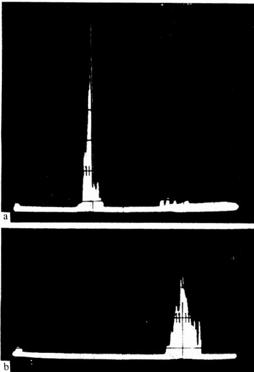
FIG. 8. Spectrograms of laser-emission modulation signals with the external reflector covered: a - Doppler beat frequency  $\Delta\nu = 9$  kHz; b - Doppler beat frequency  $\Delta\nu = 20$  kHz.
