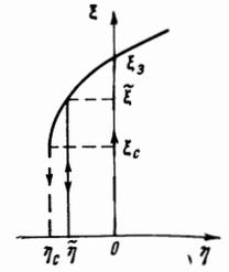
FIG. 4. Picture of the hysteresis region. Dependence of the generated power  $\xi$  on the generation parameter  $\eta$ . The dashed line with arrows indicates the region of classical hysteresis. The solid  $\eta = \tilde{\eta}$  corresponds to the pulsed regime of the laser.
