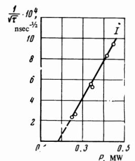
FIG. 5. Dependence of the delay time of an additional photocurrent pulse on the power density in the laser beam.  $I = 3.6$  A.
