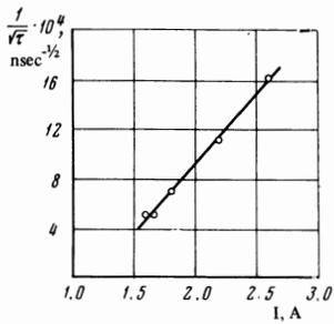
FIG. 4. Dependence of the delay time of an additional photocurrent pulse on the amplitude of the current through a crystal.  $P = 0.45$  MW.
