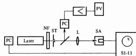
FIG. 1. Block diagram of the apparatus. PC are photocells, NF is a neutral filter, ST is a stop, L is a lens, SA is a sample, PV is a pulse voltmeter, and S1-11 is an oscilloscope.
