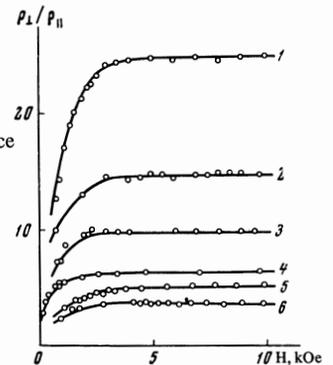
FIG. 3. Anisotropy of the resistance as a function of the magnetic field for samples with  $\rho(300^\circ\text{K})/\rho(4.2^\circ\text{K}) \sim 5 \times 10^5$ . Curves 1 for  $d = 0.10$ , 2 for 0.20, 3 for 0.33, 4 for 0.40, 5 for 0.69, 6 for 1.00 mm.
