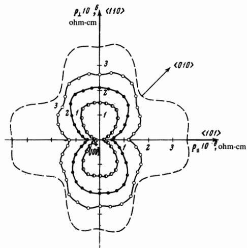
FIG. 2. Polar diagrams of the resistance  $\rho_H = 8 \text{ kOe}(\vartheta)$  for samples with  $\rho(300^\circ\text{K})/\rho(4.2^\circ\text{K}) \sim 5 \times 10^5$ . Curves 1 for  $d = 1.6$ , 2 for 0.7, 3 for 0.2 mm. The dashed curve represents data from [7].
