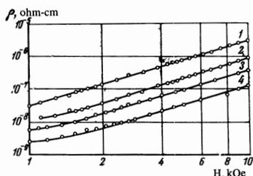
FIG. 1. Dependence of the resistance on the magnetic field for samples with the ratio  $\rho(300^\circ\text{K})/\rho(4.2^\circ\text{K}) \sim 5 \times 10^5$ . Curves 1 and 2 for  $d = 1.0$  mm are for perpendicular and parallel fields, respectively; curves 3 and 4 are for thicknesses 0.3 and 0.10 mm in a parallel field.
