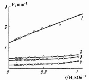
FIG. 4. Dependence of  $F$  on  $1/H$ . Curve 1 for samples with  $\rho(300^\circ\text{K})/\rho(4.2^\circ\text{K}) \sim 6 \times 10^4$  for  $d = 0.3$  mm, curves 2, 3, and 4 for samples with  $\rho(300^\circ\text{K})/\rho(4.2^\circ\text{K}) \sim 5 \times 10^4$  for  $d = 1.6, 0.7, 0.2$  mm, respectively.
