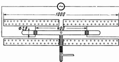
FIG. 1. Diagram of the discharge tube.
