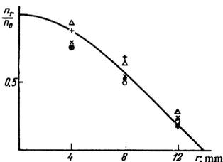
FIG. 2. Radial distribution of charged particle density in helium (p = 0.5 mm Hg, i = 25 mA): (●) H = 0, (×) H = 10 Oe, (○) H = 100 Oe, (Δ) H = 300 Oe, (+) H = 500 Oe.
