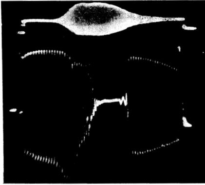
FIG. 1. Oscillogram showing the effect of rf stabilization.  $B = 1.2$  T,  $I_0 \approx 30$  mA, sample  $2 \times 2 \times 5$  mm.
