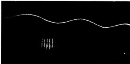
FIG. 4. Time structure of a single generator emission pulse recorded with the fast camera (period of the calibration sinusoid is 2 nsec).
