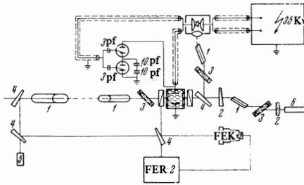
FIG. 1. Diagram of the neodymium glass laser setup for the generation of powerful ultrashort light pulses.
