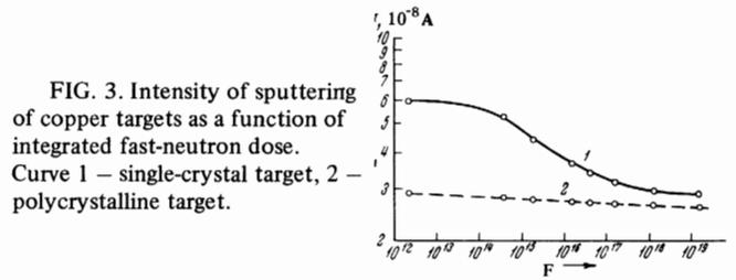
FIG. 3. Intensity of sputtering of copper targets as a function of integrated fast-neutron dose. Curve 1 — single-crystal target, 2 — polycrystalline target.
