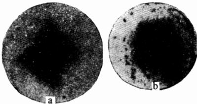
FIG. 2. Autoradiographs of deposits of sputtered atoms from the surface (a) of a single-crystal copper target, and (b) from a polycrystalline copper target.
