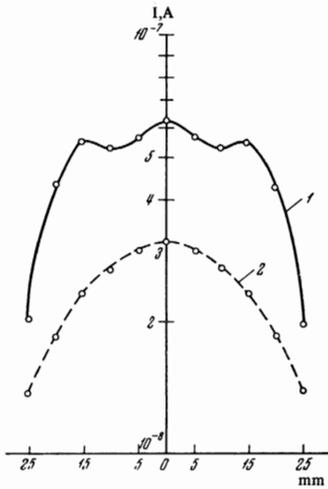
FIG. 1. Angular distributions of atoms ejected from the surface of a single-crystal copper target (curve 1) and a polycrystalline copper target (curve 2) under the action of fast neutrons.
