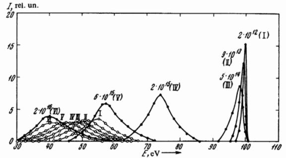
FIG. 4. Spectra of particles emitted from copper targets, as a function of the integrated fast-neutron dose. ● — Single crystal target, ○ — polycrystalline target. I —  $2 \times 10^{12}$  neutrons/cm<sup>2</sup>, II —  $9 \times 10^{13}$  neutrons/cm<sup>2</sup>, III —  $5 \times 10^{14}$  neutrons/cm<sup>2</sup>, IV —  $2 \times 10^{15}$  neutrons/cm<sup>2</sup>, V —  $6 \times 10^{15}$  neutrons/cm<sup>2</sup>, VI —  $2 \times 10^{16}$  neutrons/cm<sup>2</sup>.
