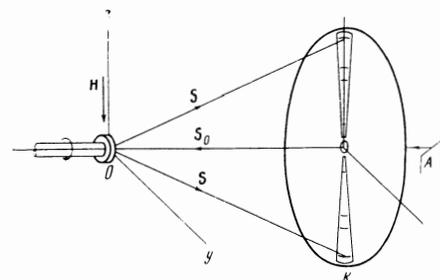
FIG. 1. X-ray diffraction setup for Dy in a magnetic field. O – sample, K – cassette with film, A – x-ray tube.
