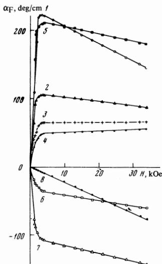
FIG. 1. Influence of external magnetic field on the Faraday effect in iron garnets of erbium (the curves correspond to different wavelengths: 1 -  $1.0 \pm 0.2 \mu$ ; 2 -  $1.5 \pm 0.2 \mu$ ; 3 -  $2.1 \pm 0.4 \mu$ ; 4 -  $4.5 \pm 0.8 \mu$ ) and holmium (5 -  $1.0 \pm 0.2 \mu$ ), gallates of yttrium (6 -  $1.0 \pm 0.2 \mu$ ) and erbium (7 -  $1.0 \pm 0.2 \mu$ ), and aluminate of terbium (8 -  $1.0 \pm 0.2 \mu$ ).
