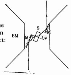
FIG. 2. Placement of the sample and of the mirrors in the gap of the electromagnetic when measuring the anisotropy of the Faraday effect: EM – electromagnetic, S – sample, M – mirrors.
