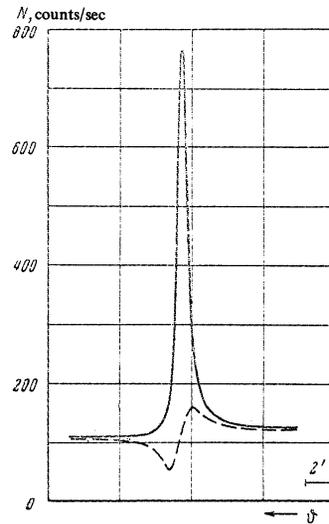
FIG. 3. Anomalous transmission of MoK $\beta$  radiation in tin. Crystal thickness—0.4 mm. (020) reflection. First-order reflection. Solid curve—crystal without impurities. Dashed curve—crystal with impurities of iron ( $\sim 10^{-4}$ ), copper ( $\sim 5 \times 10^{-4}$ ), aluminum ( $\sim 10^{-4}$ ) and antimony ( $\sim 10^{-4}$ ).
