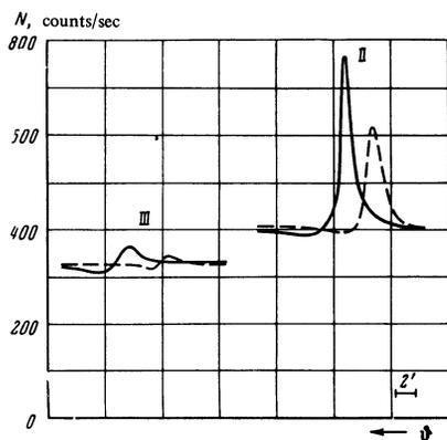
FIG. 1. Anomalous transmission of MoKβ radiation in tin. The crystal was 0.4 mm thick, (020) reflection; II, III—order of the reflection. Solid curve—T = 120°K, dashed curve—T = 293°K.
