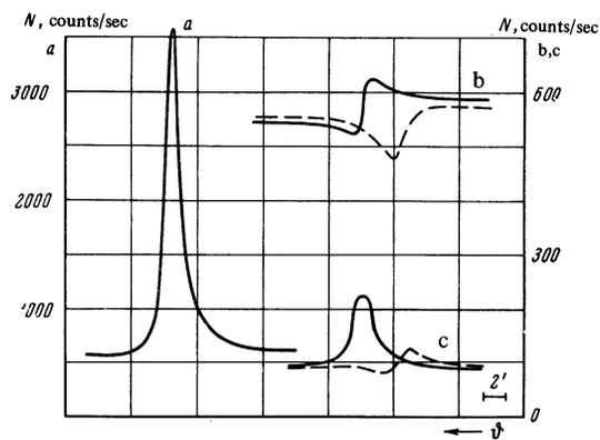
FIG. 2. Anomalous transmission of MoKβ radiation in tin. First-order reflection. Solid curves—T = 120°K, dashed curves—T = 293°K. a — (020) reflection, 0.4 mm thick crystal; b — (420) reflection, 0.4 mm thick crystal; c — (420) reflection, 0.6 mm thick crystal.
